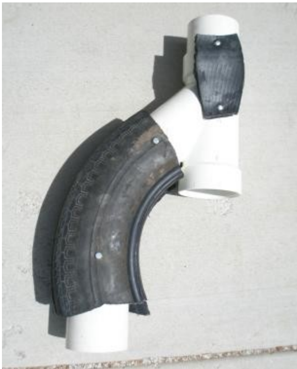
Standard WYE, 45° Street Elbow, Neck (cut from the 10'), Torso Target Extension (cut from the 10'), and Tire parts attached with bolts.
