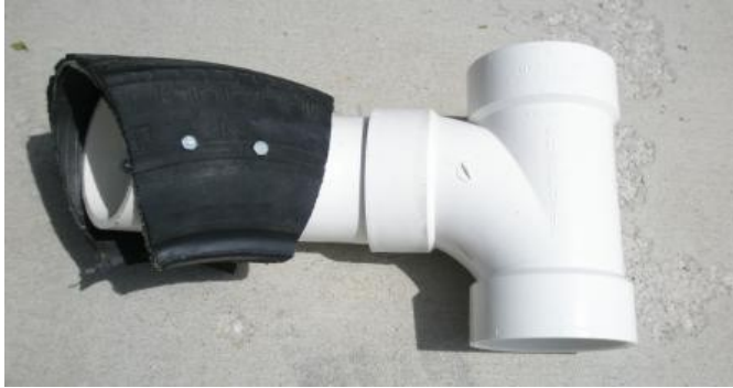
Sanitary Tee, 45° Street Elbow, Wrist Target Extension (cut from the 10'), and Tire attached with bolts.
