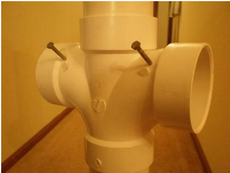
Close up of how the holes should be drilled, and the bolts inserted.
